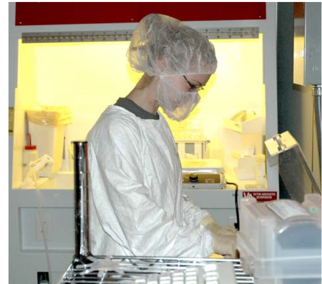
A researcher deposits a PZT film via spin-coating on 4-inch wafers in the Keck SMIL class 100 cleanroom.
