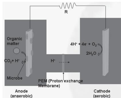
Figure 1. Microbes remove the electrons from organic matter and transfer them to the anode in the anaerobic chamber. The electrons move across the resistor to the cathode where they combine with protons, and oxygen to form water. (Figure courtesy of Jung Rae Kim)
