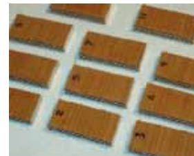
Metal joints, rather than epoxy joints, between PZT elements allow stacks to generate high power continuously
