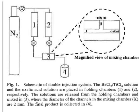
Fig. 1. Schematic of double injection system. The  $BaCl_2/TiCl_4$  solution and the oxalic acid solution are placed in holding chambers (1) and (2), respectively. The solutions are released from the holding chambers and mixed in (3), where the diameter of the channels in the mixing chamber (X) are 2 mm. The final product is collected in (4).
